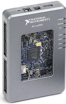
Platforma de dezvoltare National Instruments MyRIO 1900
