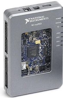
Platforma de dezvoltare National Instruments MyRIO 1900
