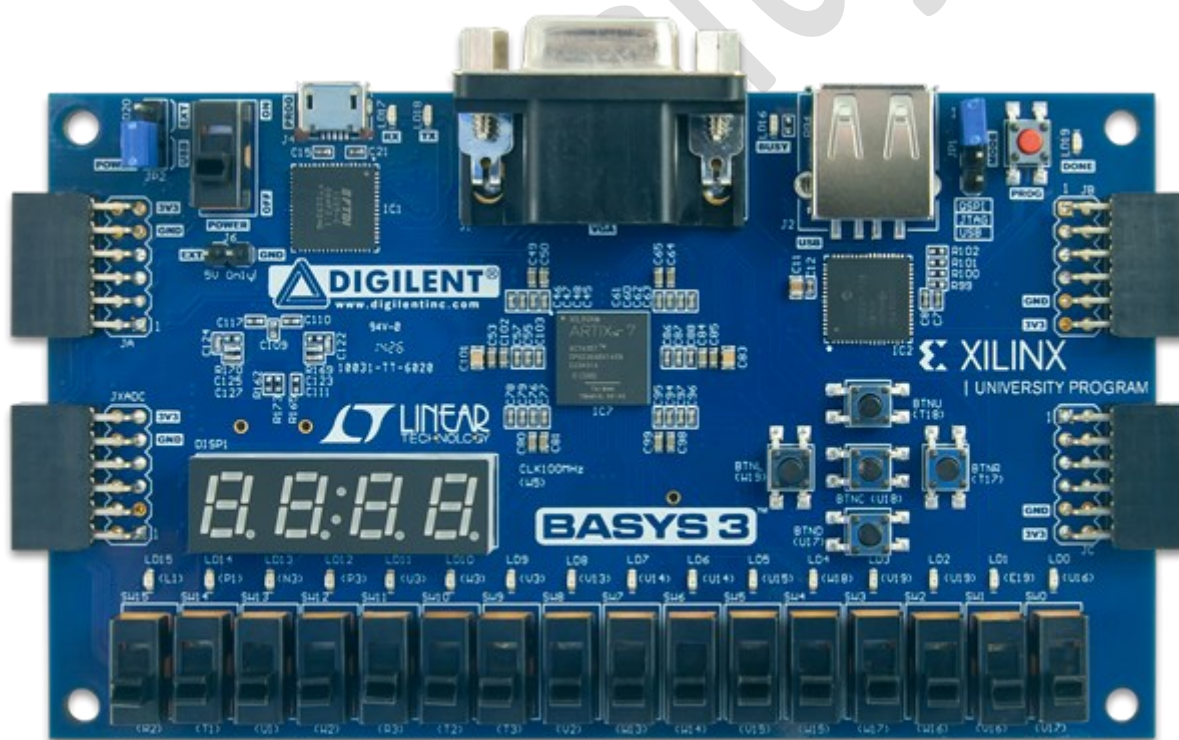
Fig. 1 - Platforma de dezvoltare Digilent Basys 3 – FPGA Xilinx Artix – 7 [2]
